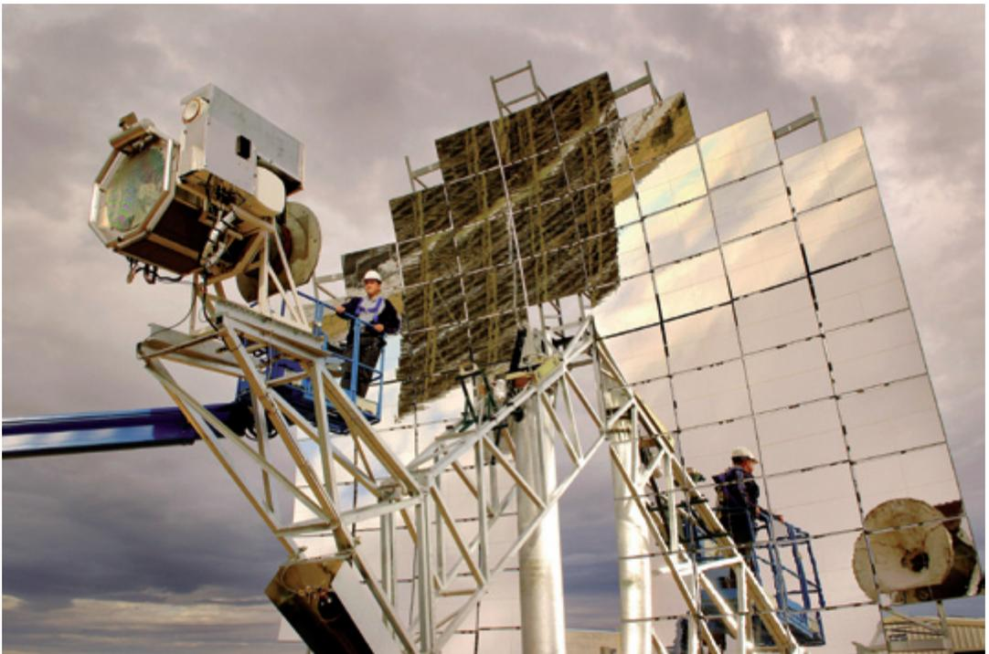
Un DISH STIRLING au Jet Propulsion Laboratory (Photo NASA JPL)
